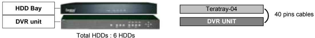
DVR unit(x2 hard disk inside) and HDD Bay(x4 hard disk inside), total is 6 HDDs.
