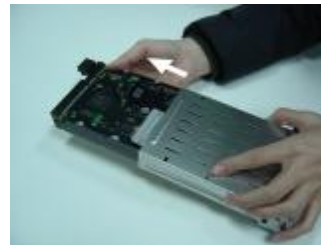
Step 5 Remove the HDD from Cartridge (refer to Picture 5).
