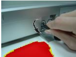
Step 2 Unlock the cabinet by turning the key anti-clockwise (refer to Picture 2).
