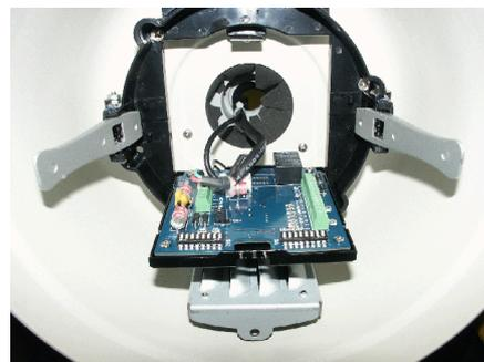
The DIP Switches are Behind the panel
